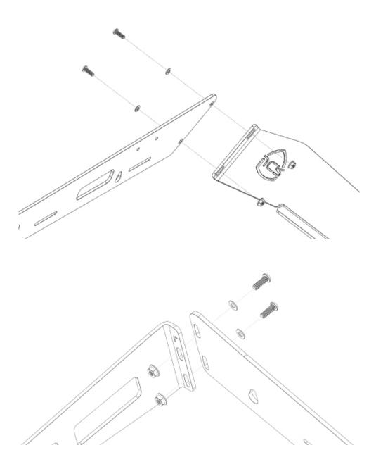
**4** Next, attach the inner mounts to the outside of the side rails using the 1/4"-20 X 3/4" button head bolts, 1/4" ID washers, and 1/4"-20 serrated flange nuts. Make sure to use the first, third and fourth sets of holes to attach your mounts. We recommend that you temporarily adjust the mount so the bolt is all the way up at the top of the slot. That way the rack is all the way up and it is easier to get it onto the roof. Tighten the bolts until the are snug, but adjustable.
