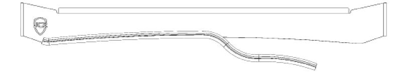
**3** Next, mount the front and rear fairings. To do this, use the1/4"-20 X 3/4" button head bolts, 1/4" ID washers, and 1/4"-20 serrated flange nuts. The front fairing will need two of each per side and the rear fairing will also need two of each per side. When mounting the front fairing, adjust it all the way up to avoid contact with the roof and leave the bolts loose enough to be able to make adjustments once it is on the roof of the vehicle.
