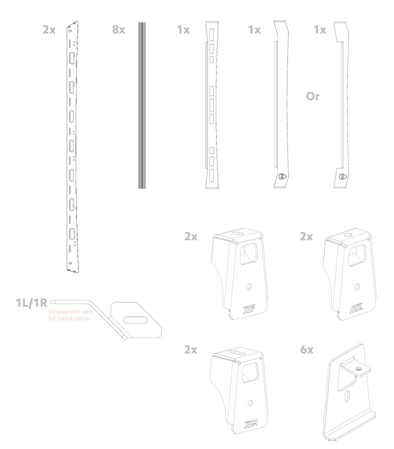
Assemble the rack on the ground. Start by mounting the crossbars between the two side rails. For this, use the 1/4"-20 X 3/4" button head bolts and the 1/4" ID washers (two per bar per side). Make sure the machined slot in the rail of the crossbar is facing up, so that you can easily add t-nuts to mount your gear.
