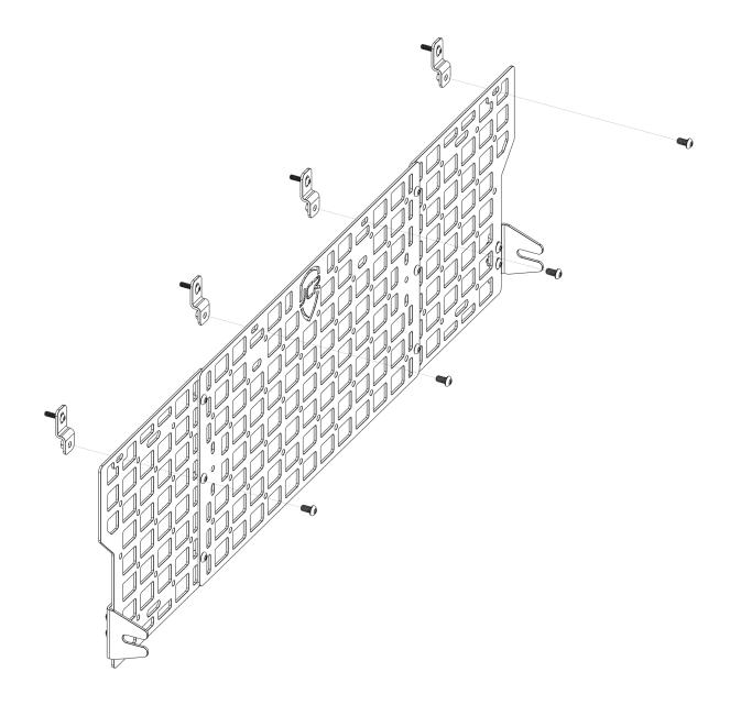
**5** Next, reinstall the tie down rings with the side mounts between the washer on the tie down bolt and the bed. Leave it loose for now.
