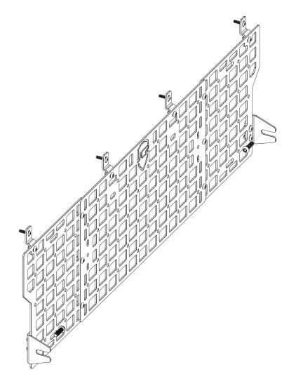
6 Finally, with everything roughly in place, position the panels however you would like them and go back and tighten all the bolts that were left loose. Try to keep the panels as close to vertical as possible.
