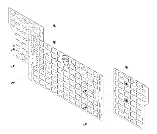
2 Next, loosely attach the side mounts to the back of the side panels using the 5/16"-18 X 5/8" bolts and 5/16"-18 serr. flange nuts. Make sure that the side with the two slots is against the back of the panel and the side with the one slot is sticking out towards the tailgate. Then, remove the small swiveling tie down rings by the front of the bed from both sides. These will be used later to fasten the panels into place.
