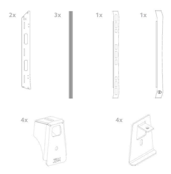
1 Assemble the rack on the ground. Start by mounting the crossbars between the two side rails. For this, use the 1/4"-20 X 3/4" button head bolts and the 1/4" ID washers (two per bar per side). Make sure the machined slot in the rail of the crossbar is facing up, so that you can easily add t-nuts to mount your gear.
