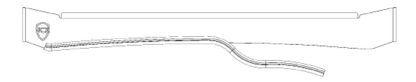
3 Next, mount the front and rear fairings. To do this, use the 1/4"-20 X 3/4" button head bolts, 1/4" ID washers, and 1/4"-20 serrated flange nuts. The front fairing will need two of each per side and the rear fairing will also need two of each per side. When mounting the front fairing, adjust it all the way up to avoid contact with the roof and leave the bolts loose enough to be able to make adjustments once it is on the roof of the vehicle.
