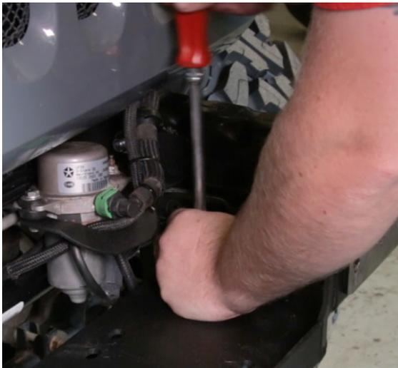
**8** Install the winch to the winch tray and run your wiring into the engine bay
