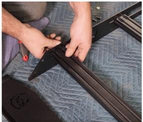
2 Install the edge trim on the front and rear fairings. Loosely install the trim on the front fairing from point to point and trim the excess with a pair of tin snips. The leftover will be installed in the center of the rear fairing.
