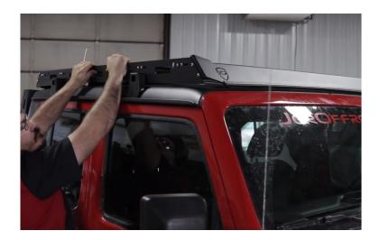
Position the rack from front to back on the roof. A good rule of thumb is to place the rear fairing at the seam in the back of the hardtop. Install the outer mounting brackets, leaving them loose until you have all of them started. We recommend using red Loctite on the side outer bracket bolts.
