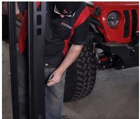
Bolt the fairings on the rack, using the same 3/4" button head bolts and washers as the crossbars, with the addition of flange nuts on the inside (3 per side for the front fairing, 2 per side for the rear). For now, position the fairings up as high as they will go and snug the bolts. We will adjust them down once the rack is on the roof.
