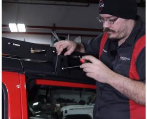
Adjust the rack up and down at each mount to level the rack. Then tighten up all of the mounting brackets. Adjust the fairings down firmly against the roof. This will prevent them from flexing at higher speeds.
