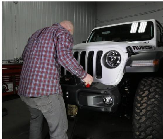
**10** Next, tighten the bumper using the factory hardware. To tighten the inside bolts you may have to use an extension. Use a 5/8 socket to tighten the bolts we used earlier to hold the winch plate in place as shown in picture C and D.
