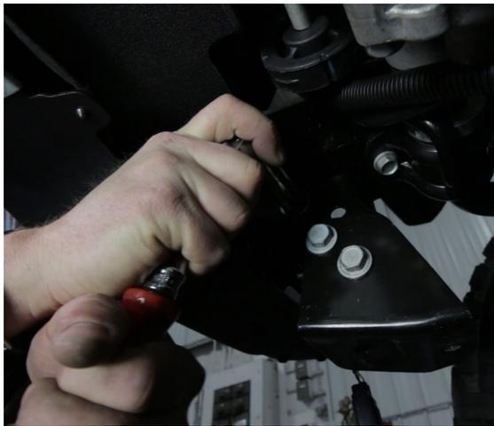
**11** After the bumper is tight, remove the jack as shown in picture A. Then, connect the factory fog light harness that we disconnected earlier in the installation as shown in picture B. Finally, reinstall the factory skid plate. Hand tighten the bolts and then go back and tighten them down with a 13mm socket.
