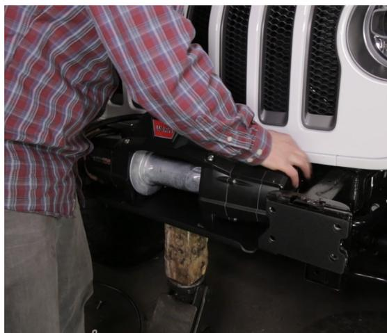
**7** Next, remove the plastic blockoff plate on the factory steel bumper by pushing on the 6 clips holding the plate to the bumper as shown in picture A. Take the bracket that we provide and hold it on the outside of the bumper as shown in picture C. Bolt the bracket to the bumper with the button head hardware (4 bolts) provided in the kit as shown in picture D.
