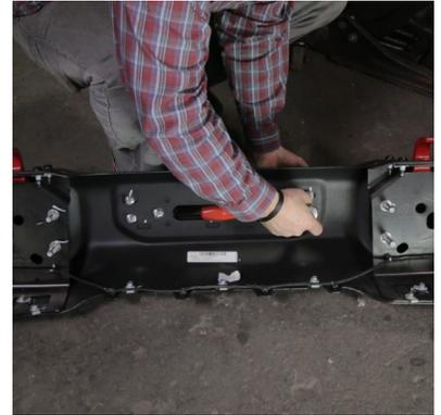
**Note:** If the frame horn sticks out further than our bracket you may have to trim the frame horn to the edge of our bracket. This only applies if you have a Warn Zeon or another large winch.
