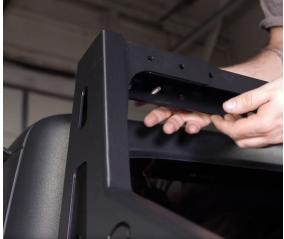
Position the Chase Rack where you want it front to back on the bed and fully tighten the bedside mounting brackets using a 1/2" socket or wrench. Ensure that the clamping brackets (if you are using them) are up as far as they will go behind the bedside.
