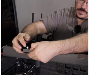
**3** Place the side panel on the bedside, slide the clamping brackets up behind the edge of the bed rail as high as you can and snug up the nuts by hand to hold it in place.
