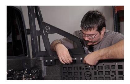
6 Adjust the crossbar to align the side panels with the side of the cab. Tighten them down with a 3/16" allen key or bit.
