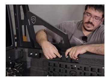
4 Now that both side panels are installed, place the crossbar between the two. Loosely install it with four button head bolts and flange nuts per side.
