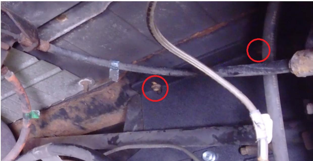
**5** Using a floor jack, transmission jack or a friend, lift the new skid into place, being careful to line up the 3 holes in the skid to the 3 carriage bolts previously installed. Loosely tighten flange nuts to secure.
