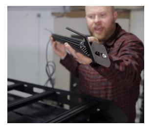
**9** Slide two t-nuts into each slot on the front crossbar. Bolt the light bar mounting brackets to these t-nuts using the 1/4" bolts and washers. Position your light bar and tighten down all of the hardware.
