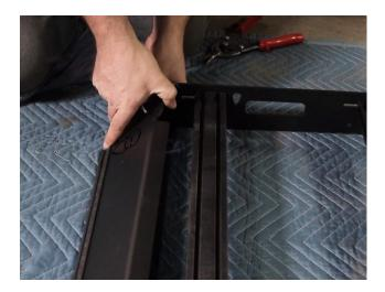
**4** Now install the mounts using the same hardware as the fairings. All of the mounts will be the same. Install them on the inside of the side rails, with the mount bending outward.
