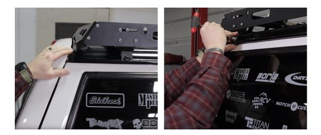
7 Adjust the rack up and down at each mount to level the rack. Then tighten up all of the mounting brackets. Adjust the fairings down firmly against the roof. This will prevent them from flexing at higher speeds. Dirt/debris can get stuck in the edge trim over time and could wear on your paint. You can us 3M clear protection film on your roof under the fairings to protect it.
