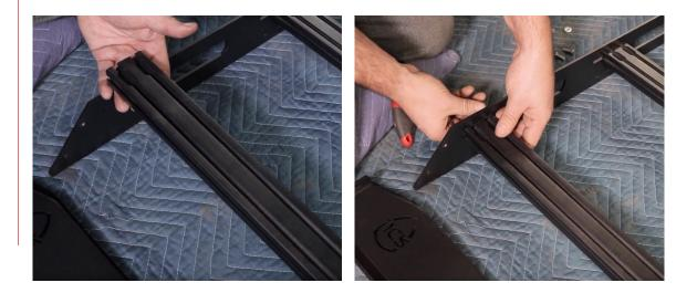
2 Install the edge trim on the front and rear fairings. Loosely install the trim on the front fairing from point to point and trim the excess with a pair of tin snips. The leftover will be installed in the center of the rear fairing.
