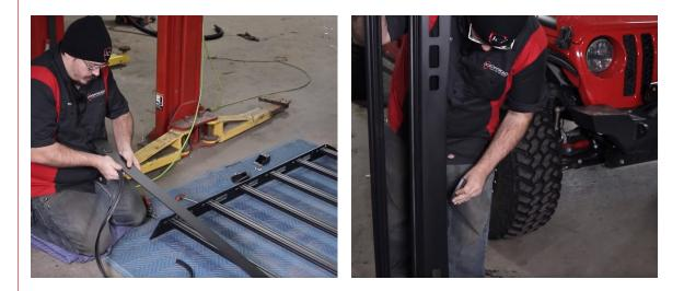
**3** Bolt the fairings on the rack, using the same 3/4" button head bolts and washers as the crossbars, with the addition of flange nuts on the inside (3 per side for the front fairing, 2 per side for the rear). For now, position the fairings up as high as they will go and snug the bolts. We will adjust them down once the rack is on the roof.
