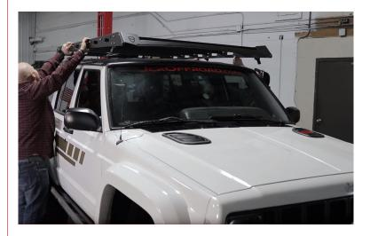
6 Position the rack from front to back on the roof, as pictured. Install the outer mounting brackets, leaving them loose until you have all of them started. We recommend using red Loctite on the side outer bracket bolts. You could also put rubber or liquid electrical tape on the outer mounts to keep them from marring your paint.
