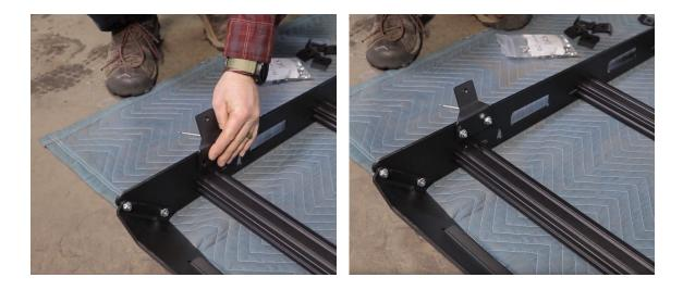
**5** With the help of a friend, place the rack up on the Jeep with the mounts sitting in the drip rails.
